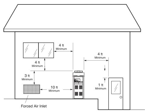
Figure 6. Outdoor Installation Clearances.
